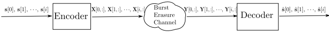
Fig. 1. System under consideration. Each \mathbf{X}[i, :] denotes a (channel) macro-packet consisting of M channel packets ( \mathbf{x}[i, 1], \dots, \mathbf{x}[i, M] ). One source packet arrives at the start of each macro packet. The channel erases up to B consecutive channel packets. Each source packet needs to be reconstructed with a delay of T macro packets.
